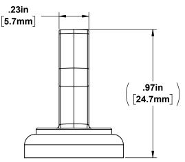
CULUSTED US **UL LISTING** Magnetic Cable Holder 3/4" Positioning Devices ANSI/UI Mechanical 1565 TYPE 21 E359769 Tensile Strength: 10 LBS. (45Ň) CSA-C22.2 No. 18.5 CAN No Load Rating ALL TESTING PERFORMED USING 3mm MIN. THICK 1008-1010 STEEL PLATE
