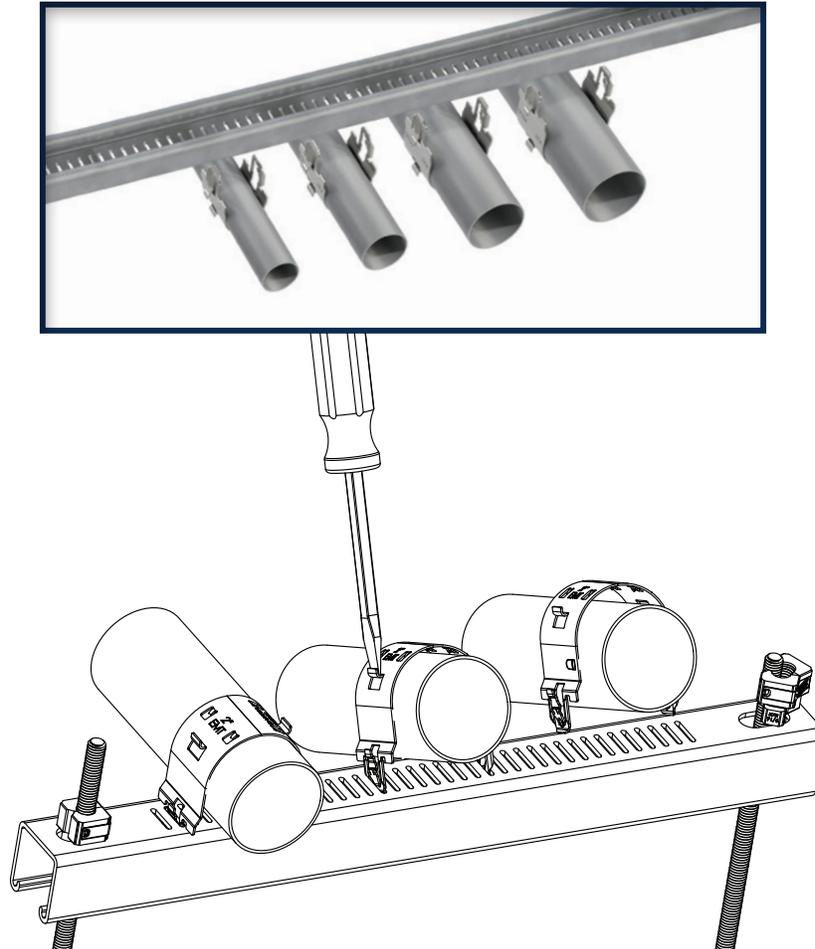
To install, insert the tabs of the Smart-Clamp into the slots
